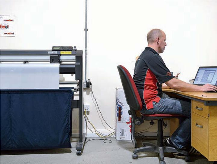
The process begins with the film kit cut to size and shape in-house on a graphics plotter
