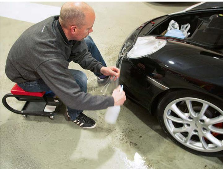
Each individual piece of film requires a slip and fix solution to bond to the car's panels
