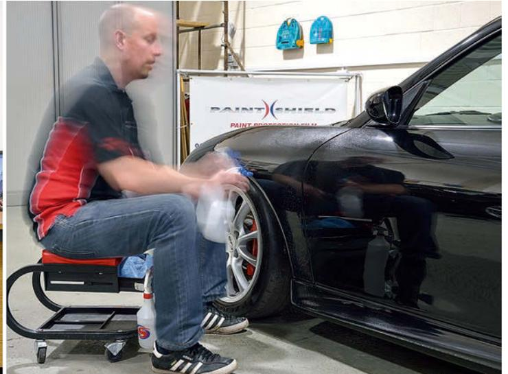
Every panel is cleaned and prepared so no blemishes are trapped before film application
