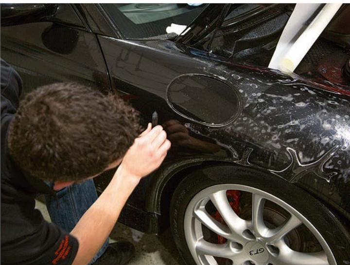
The fix solution reacts to the adhesive which then bonds the film to the body panel
