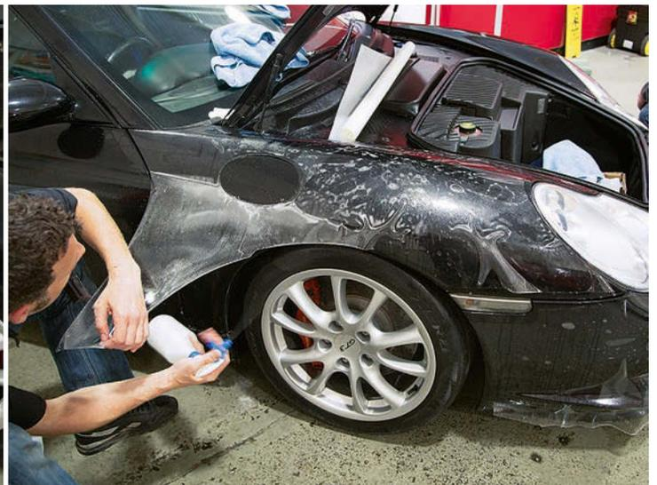
A slip solution allows the fitter to position the film precisely on the panel before it's fixed
